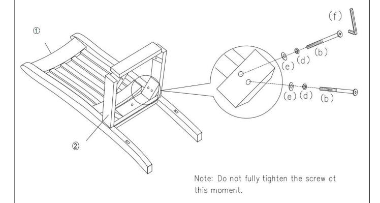
Fix the base frame (2) to the chair back (1) through the corner blocks of base frame (2) with Allen bolts (b),spring washers (d) and steel washers (e).
