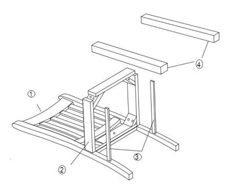
Insert the stretchers 3 into the leg of chair back 1. Position the front legs 4 onto stretchers 3 and base frame 2.
