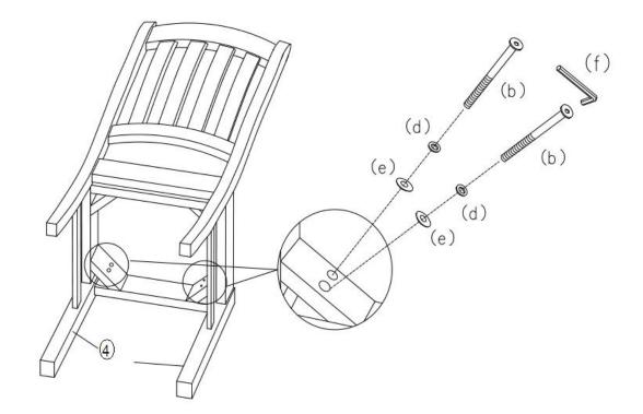
Fasten legs 4 to corner block with Allen bolt (g), spring washer (d) and steel washer (e).
