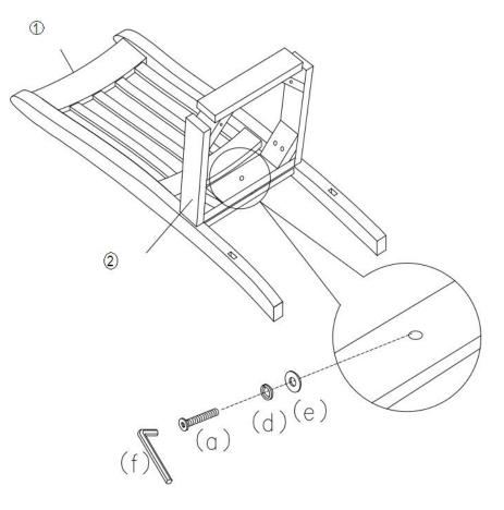
Fasten the base frame 2 to the chair back 1 with Allen bolt (a),spring washer (d) and steel washer(e).
