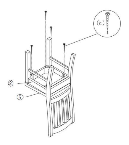
Fasten the seat (5) to the base frame (2) with wood screws (c). Carefully turn the chair over. Repeat with the remaining chair.
